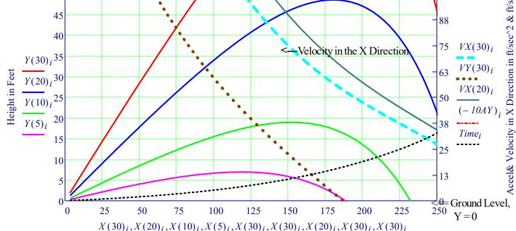
Spud Trajectories, Velocities & Accel w Air Drag at Angles of 40,30,20,10 deg
